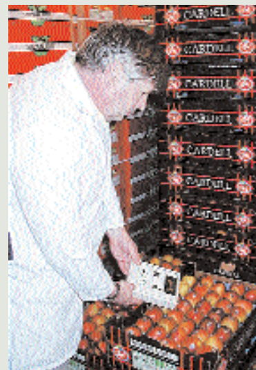
David Bishop, ICA's Technical director testing the ethylene level with the new ICA56 Ethylene analyser in a cold store constructed by ICA in Kent.
